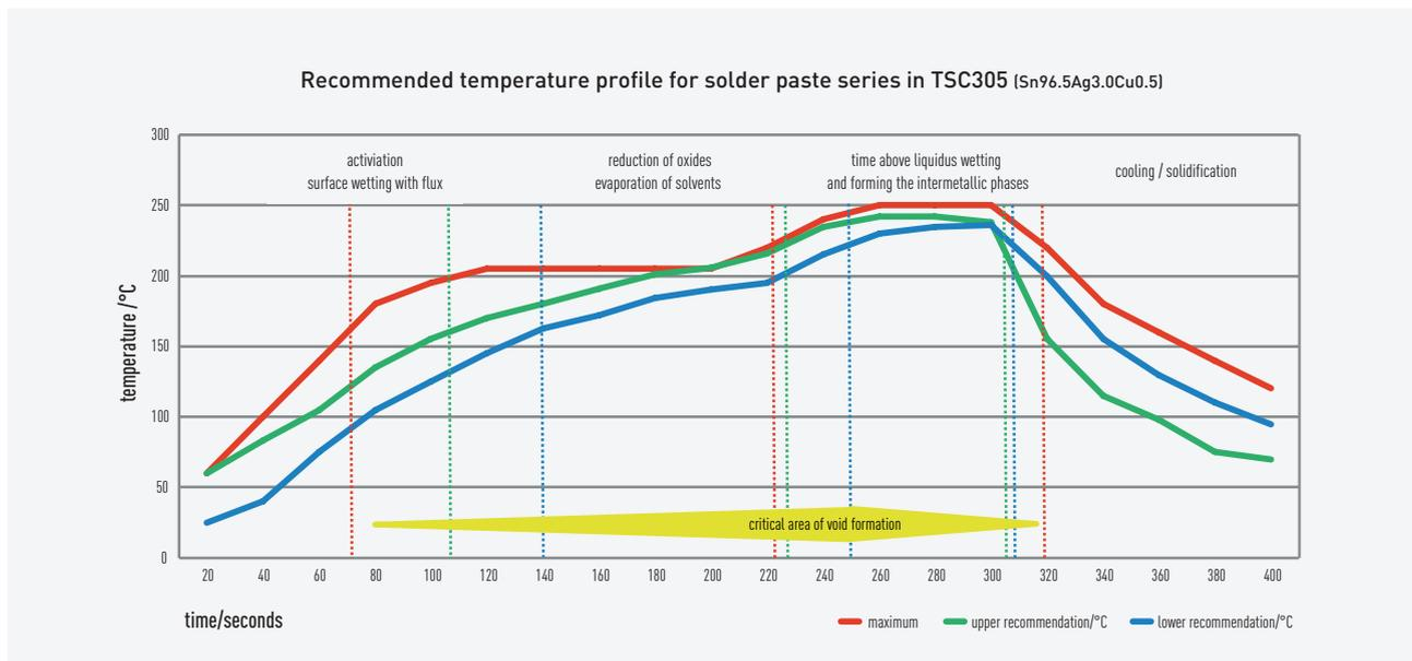
Newly developed solder pastes can often be easily integrated into existing processes. Nevertheless, depending on the PCB and component configuration, it may be necessary to make minor changes to the temperature profile to achieve the desired performance of the flux. As a good starting point, the middle of the process window at 25 °C for 40 to 60 seconds above the melting point (liquidus) is satisfactory and generally gentle on the components.
