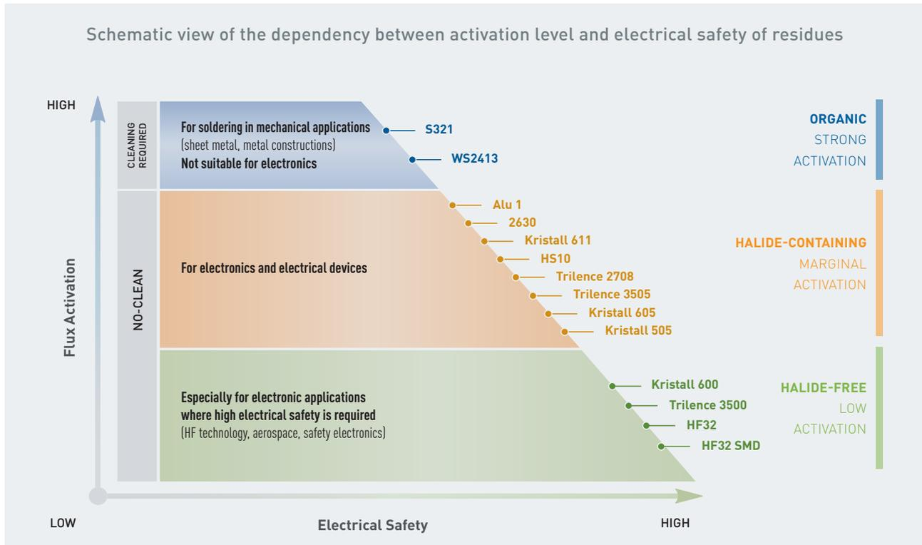
This illustration shows the relation of the flux activation to the electrical safety of the flux residues after the soldering process. For example, good electrical safety can be achieved with Kristall 611 containing an activated flux – as a No-Clean flux even without cleaning after the soldering process.
