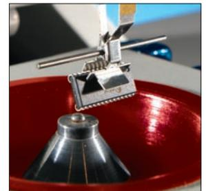
pass/fail) are identical to those offered for components. Test results can also be displayed as a series of colour-coded wetting force curves, with failed components highlighted on the results display screen. Graphs and test data can be sent direct to a suitable parallel printer and/or stored on disk.
