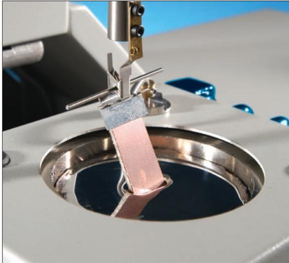
The MUST System 3 is a high precision solderability tester for surface mount (SM) and through-hole (TH) components, as well as PCB pads and plated through-holes (PTHs or vias) on bare boards. It is also ideal for the laboratory testing of fluxes and other soldering materials.
