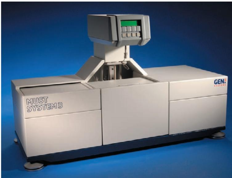
The solderability of a Printed Circuit Board (PCB) or component’s metallic terminations is a critical parameter in any soldering operation because it represents the likelihood of that termination forming a good alloy with the solder and a high quality solder fillet.
