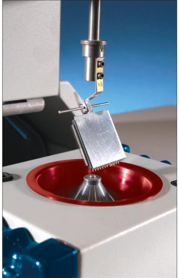
This technique produces a larger wetting force for analysis and also allows small surfaces, such as 0402 or smaller terminations, including 0201s, and the individual leads on a multi-leaded component, to be tested. As before, the specimen is fluxed, dried and suspended from the measuring head of the Wetting Balance.
