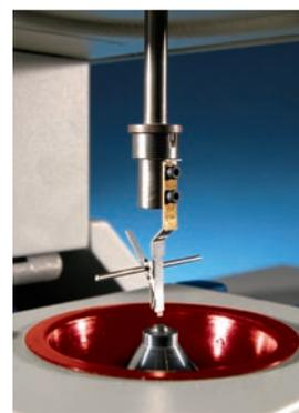
well the solder wets it and thus its solderability. In simple terms, the greater the solderability, the higher a meniscus will climb, which can be measured as a change in the vertical force acting on the suspended specimen (Figure 1).
