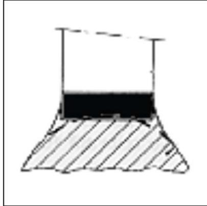
**Figure 13 1206 Capacitor immersed 0.1 mm into a 200 mg globule**
